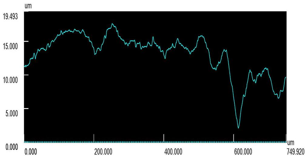
**Fig. 9.** Distribution of depth values for a crack fragment 750  $\mu\text{m}$  wide according to laser confocal microscopy data.
