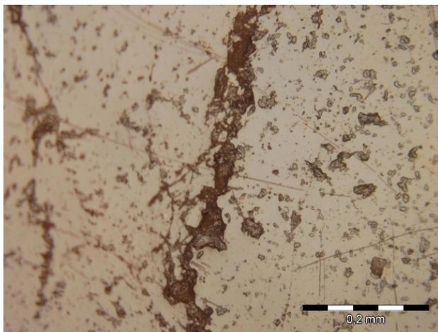
**Fig. 4.** View of a microcrack in a granite sample according to optical microscopy data.
