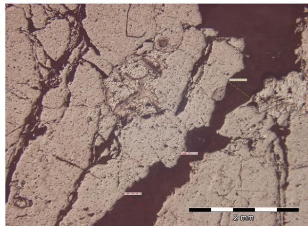
**Fig. 7.** View of a separate fragment of a crack in granite according to optical microscopy data.
