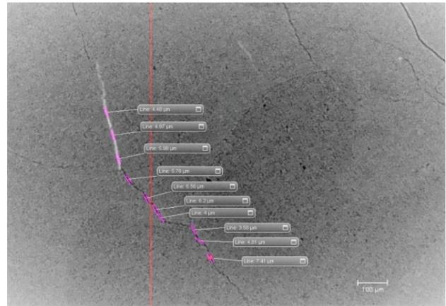
**Fig. 5.** Type of microcrack and assessment of the size of its opening based on X-ray computed microtomography data.
