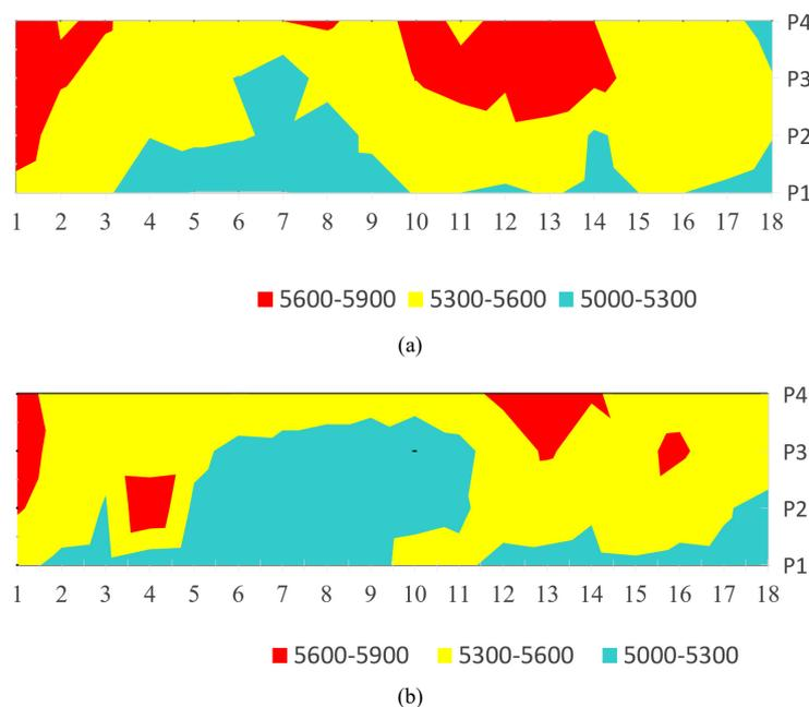
**Fig. 3.** Distribution of longitudinal wave speed values (m/s) in a granite sample before (a) and after (b) dynamic impact.
