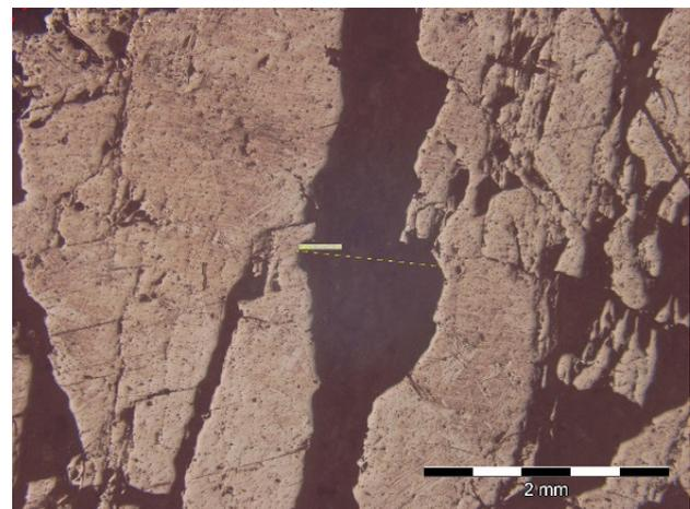
**Fig. 6.** View of a separate fragment of a crack in granite according to optical microscopy data.
